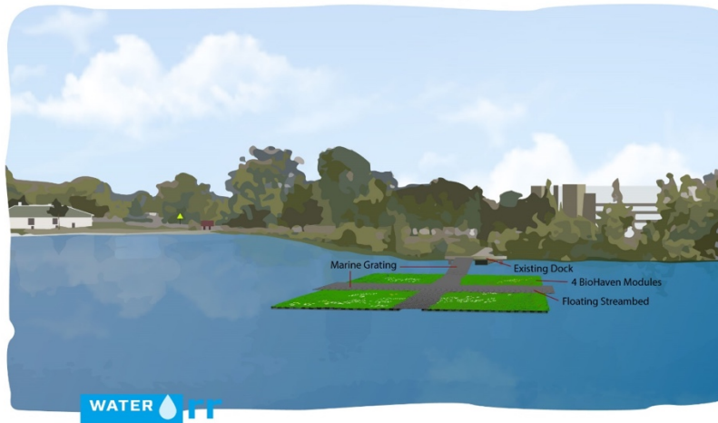
Figure 2b. Possible configuration of a Science Island with BioHaven StreamBed in The Sac
