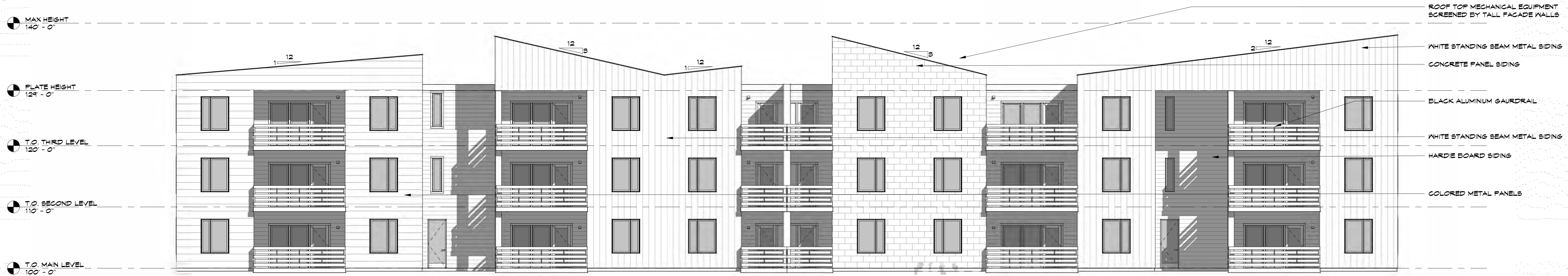
4 ELEVATION - 36 UNIT BUILDING 1/8" = 1'-0"
